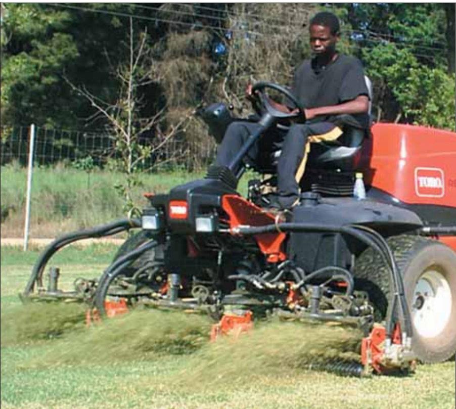
ABOVE: The fairways are cut using this special hydraulically controlled, ride-on mower.
